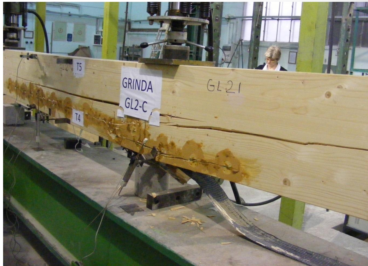
Fig. 9. Failure mode aspects of the items tested
